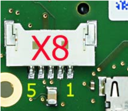
Figure 17: Backlight and Display Control Connector X8
