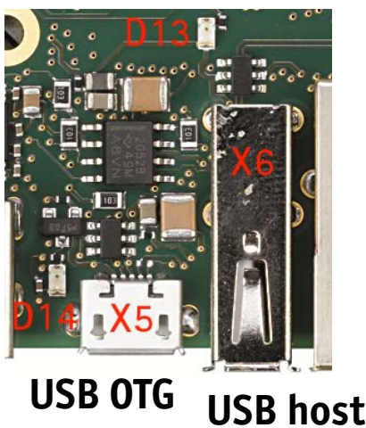
Figure 8: Components supporting the USB Interfaces
