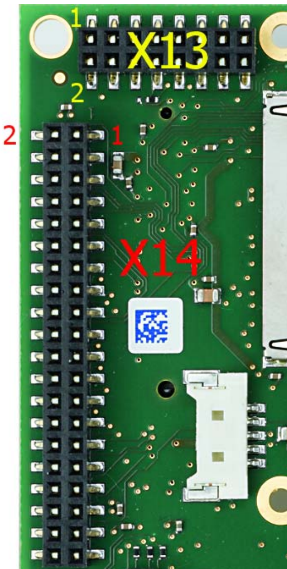
Figure 21: Audio/Video Connectors (X13 and X14)
