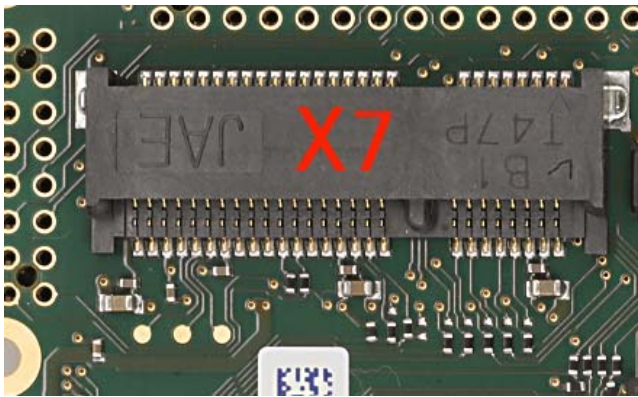
Figure 12: PCIe Interface at Connector X7
