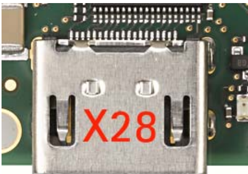
Figure 15: HDMI Interface Connector X28
