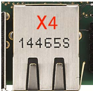
Figure 7: Ethernet Interface at Connectors X4
