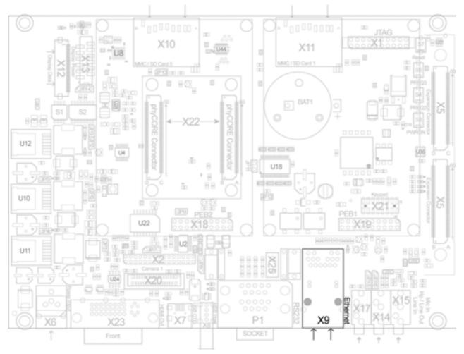
Figure 25: Ethernet Interface at Connector X9
