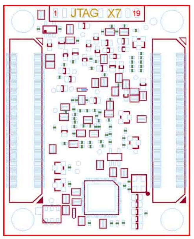
Figure 10: JTAG Interface at X7 (bottom view)
