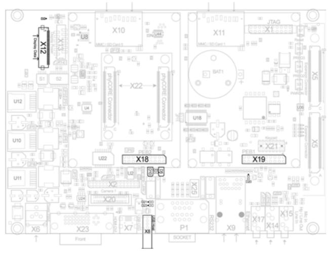
Figure 26: Components supporting the USB Host Interface
