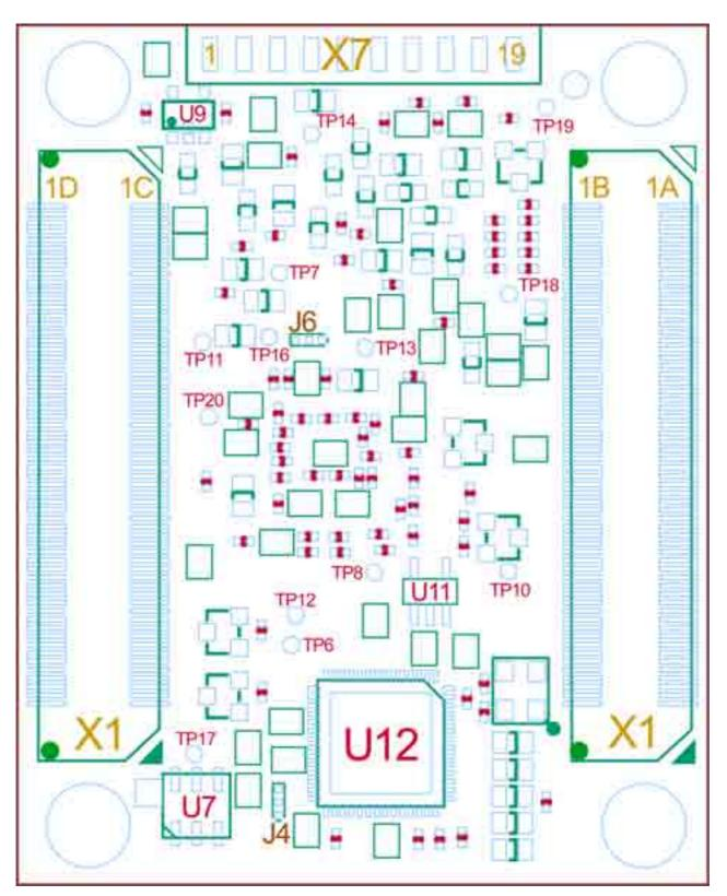
Figure 3: Bottom view of the phyCORE-OMAP44xx (connector side)
