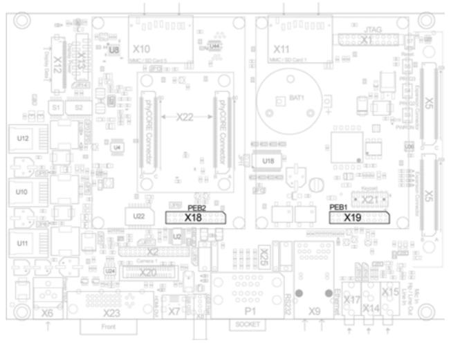
Figure 40: Extension Connectors X18, X19
