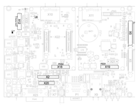
Figure 35: I<sup>2</sup>C Connectivity (top view)
