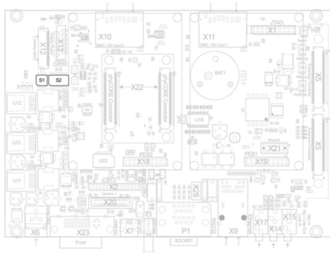
Figure 43: Boot Mode Selection Switches S1 and S2
