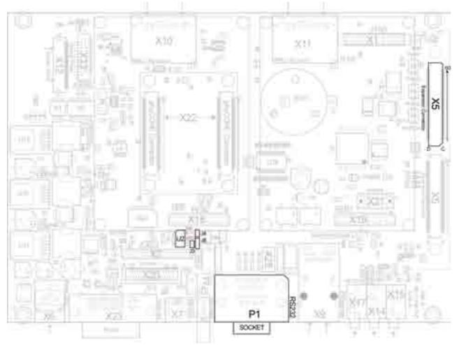
Figure 23: RS-232 Interface Connectors (P1, X5) and Jumpers
