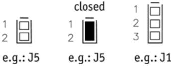
Figure 5: Typical Jumper Pad Numbering Scheme
