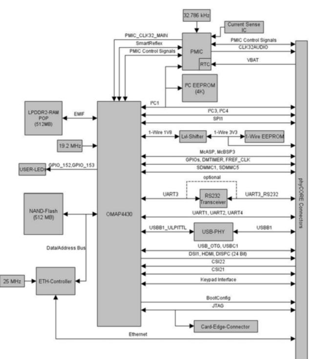
Figure 1: Block Diagram of the phyCORE-OMAP44xx
