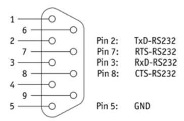
Figure 24: RS-232 connector P1 Signal Mapping
