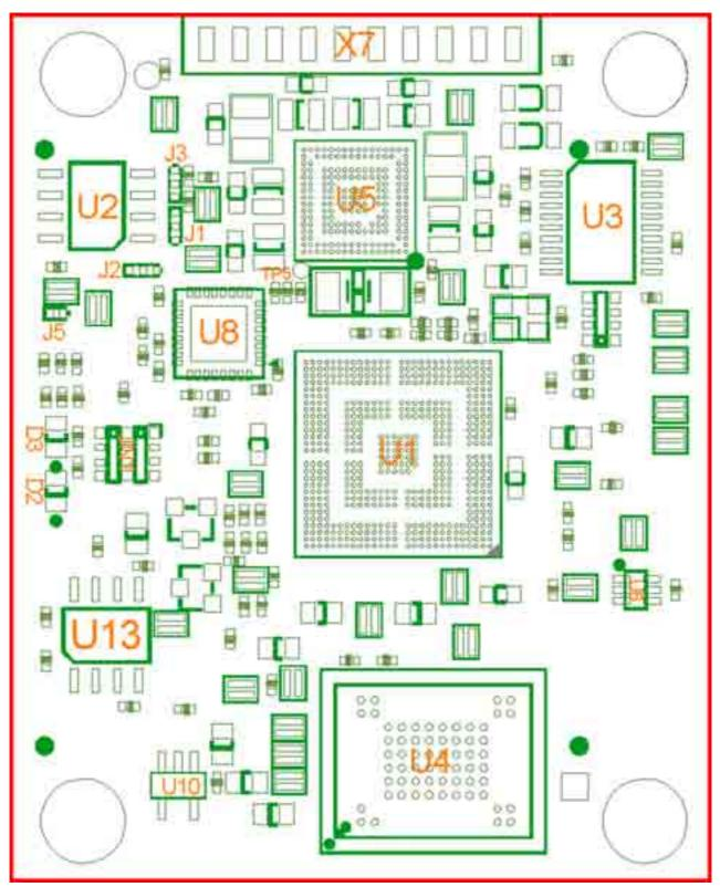
Figure 2: Top view of the phyCORE-OMAP44xx (controller side)
