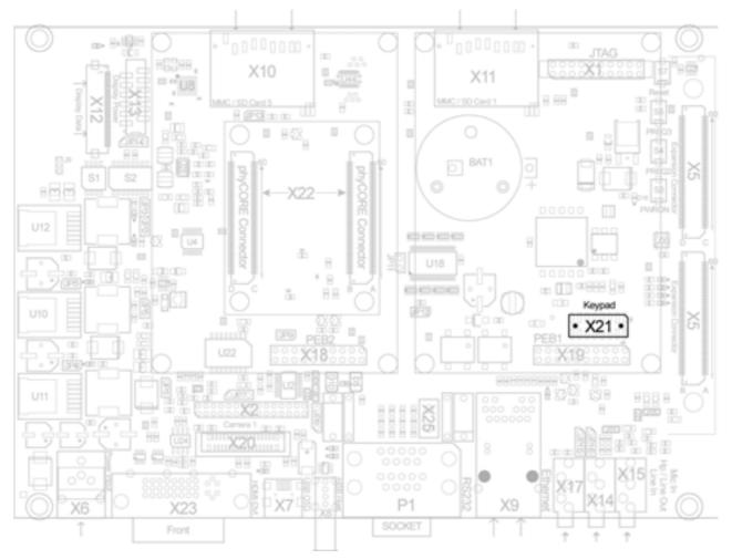
Figure 46: Keypad Connector X21
