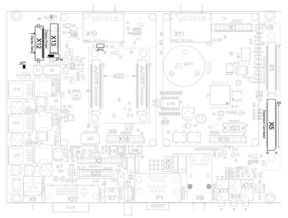
Figure 28: Display / Touch Connectivity (X12, X13)(top view)
