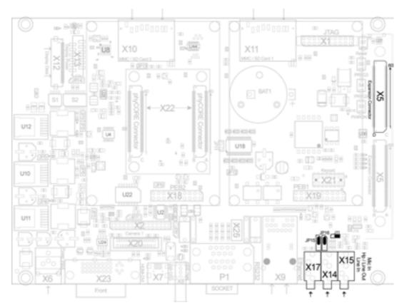
Figure 33: Components supporting the Audio Interface at connectors X5, X14, X15 and X17 (top view)
