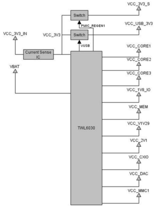
Figure 8: Power Supply Diagram
