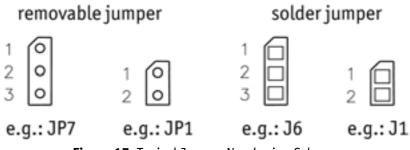
Figure 17: Typical Jumper Numbering Scheme
