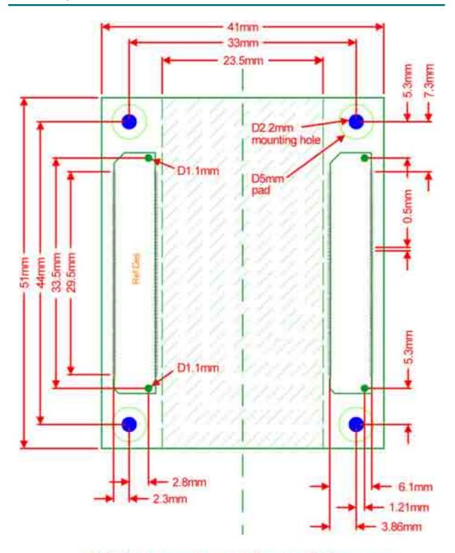
shaded area represents space to place noncritical components (no RF emission, no thermal radiation, etc.) underneath the module
