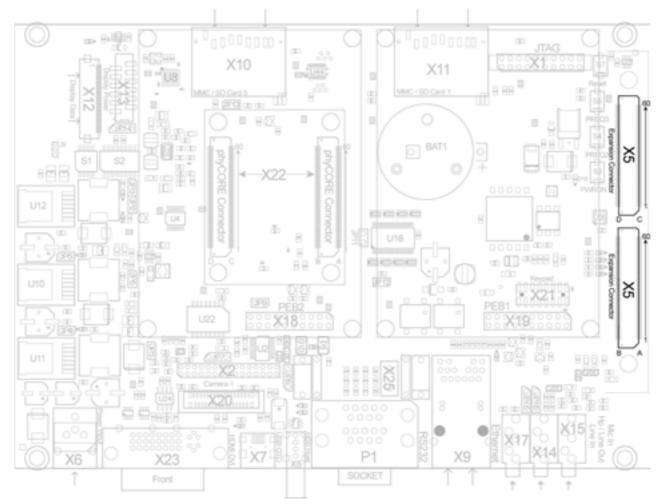
Figure 47: Expansion Connector X5
