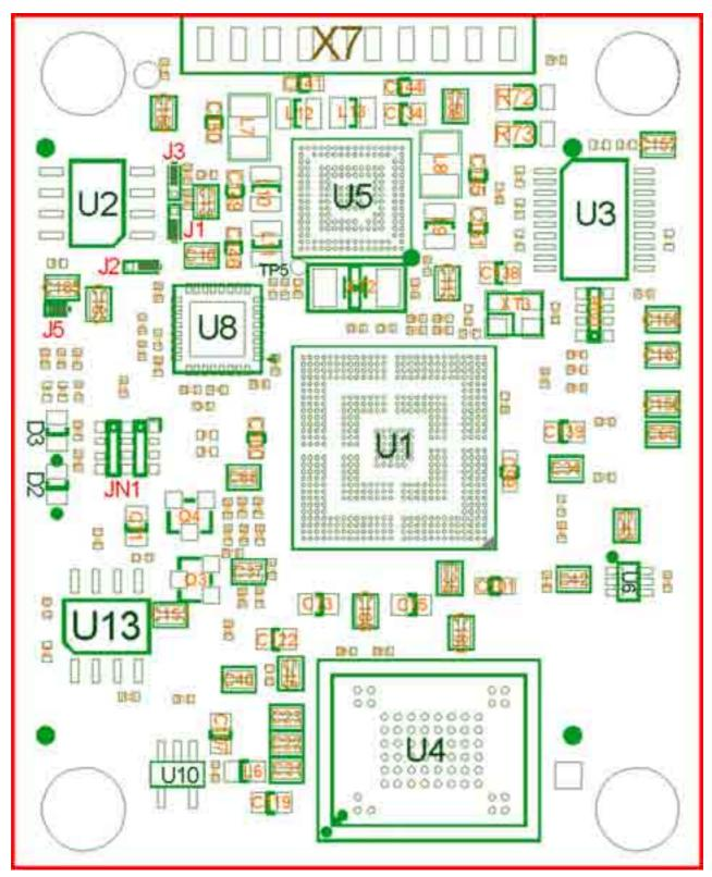
Figure 13: phyCORE-OMAP44xx Component Placement (top view)
