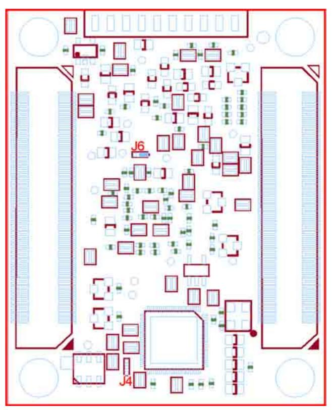
Figure 7: Jumper Locations (bottom view)
