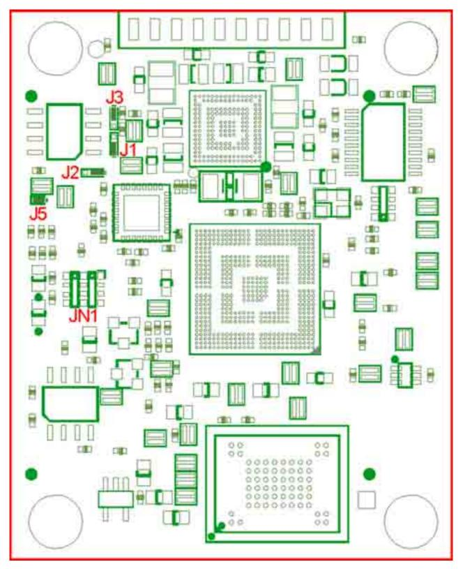
Figure 6: Jumper Locations (top view)
