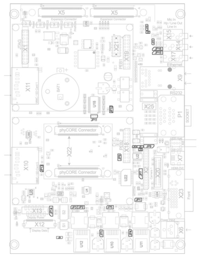
Figure 18: phyCORE-OMAP44xx Carrier Board Jumper Locations (top view)
