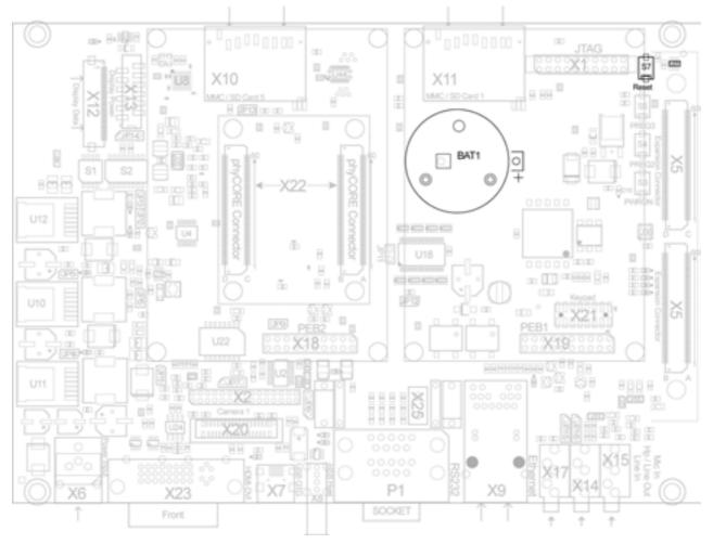
Figure 44: System Reset Button S7
