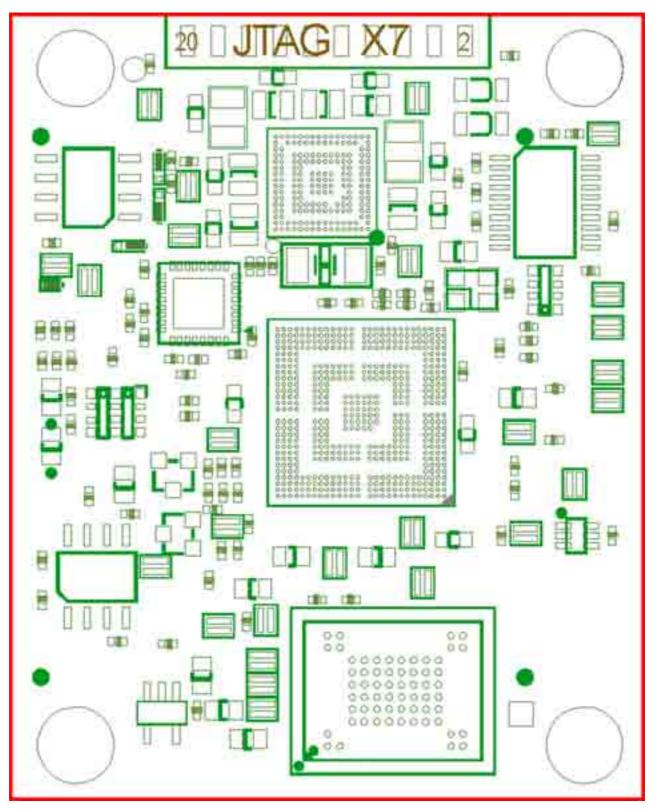
Figure 9: JTAG Interface at X7 (top view)
