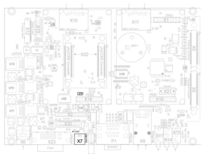
Figure 27: USB OTG Interface at Connector X7
