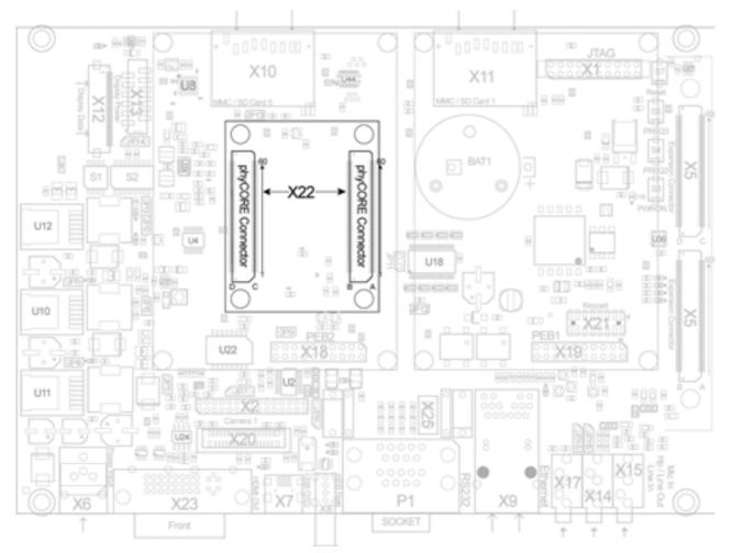
Figure 20: phyCORE-OMAP44xx SOM Connectivity to the Carrier Board
