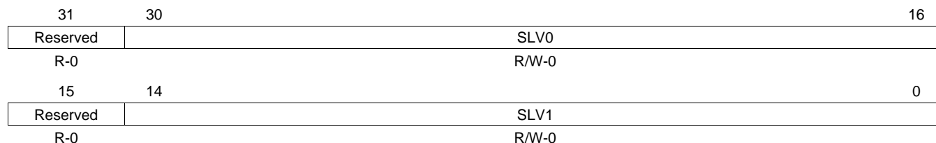
Figure 10-25. Vertical Line - Settings for the Starting Pixel Register (VERT_START)
