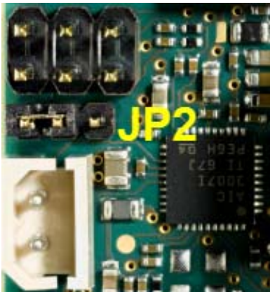
Figure 23: Audio Codec Disable Jumper JP2
