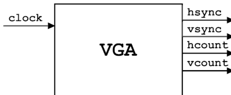
Figure: Shows a high-level view of the first VGA driver to create.
