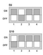
Note: Be careful when changing these switches as the S9 and S10 packages are rotated 180° off of each other so the switches will be on opposite sides for both OFF and ON and count 1-4 in different directions.
