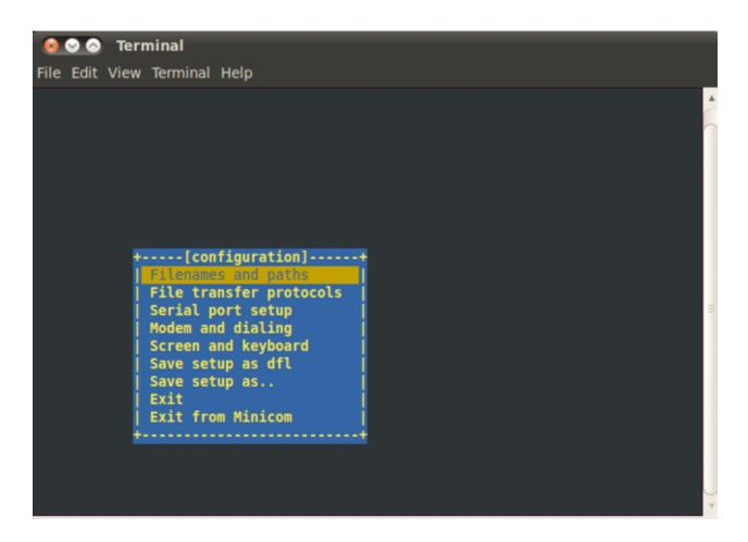
Navigate to "Serial port setup" in the Minicom main menu and modify line A - Serial Device : to read /dev/ttyS0 and line E - Bps/Par/Bits : to have a speed of 115200 and 8-N-1 (8N1) for the stop bits:
